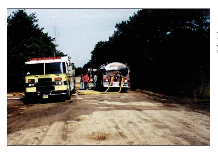
Tanker shuttle drill using Turbodraft at a fill site that was not accessible for typical drafting techniques.
