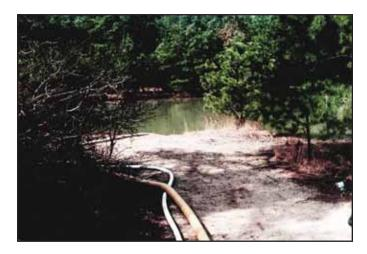
Due to soft sand and trees the engine was not able to be positioned to allow for drafting at this location. With the Turbodraft we were able to access the water source from approximately 100 ft away and fill tankers at a rate of 600 gpm.
