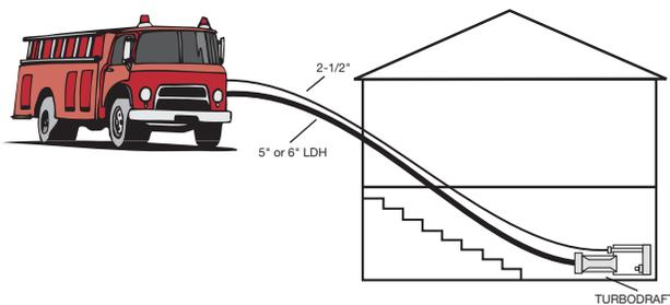
TurboDraft can also be employed in emergency flood situations. TurboDraft's ability to transfer large volumes of water in a short amount of time makes it a critical piece of equipment for dewatering basements and other low-lying areas where water collects.
