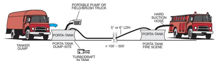
TurboDraft can be used in conjunction with a portable pump to provide constant flow between remote tanks and fire scene supply tank. Flow from the remote tanks can be controlled by a gate valve in the 5" or 6" supply line. If discharge line is blocked, supply line flow is discharged into portable tank and recycled.
