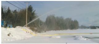
Outfitted with an ice strainer, the TurboDraft CS eductor provides quick access to frozen static sources. TurboDraft's ability to transfer large volumes of water in a short amount of time makes it a critical piece of equipment.
