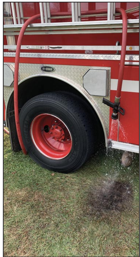
13 Be mindful of the heat generated by the high engine rpm during a TurboDraft operation and take the necessary steps to establish an exposure line.
