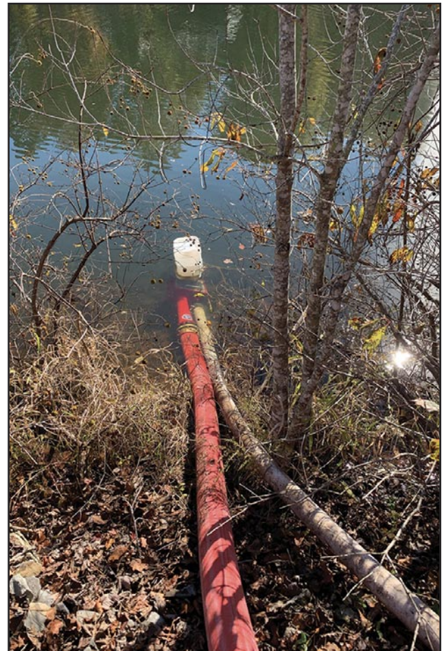
7 The easiest way to deploy the device is to attach some sort of float to the eyelet on the device and toss it into the water.
