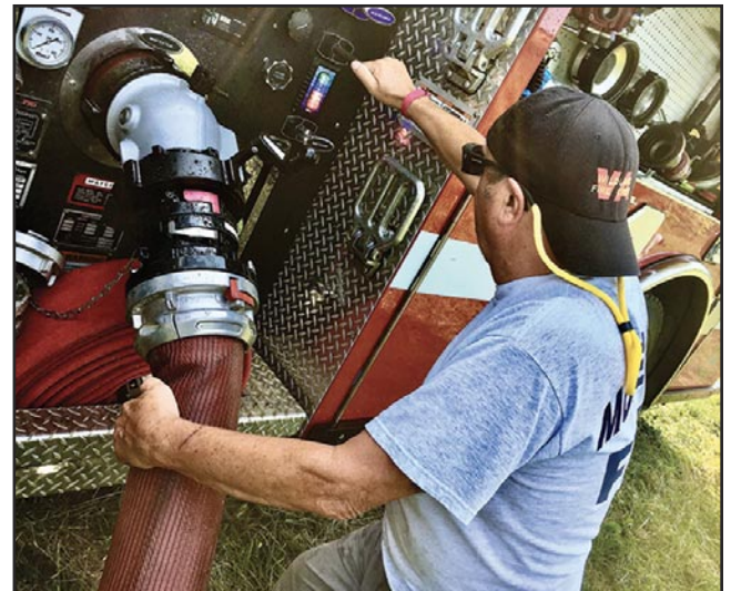
10 The TurboDraft reaches its peak flow capability once the supply line begins to get soft enough to "squeeze." It is imperative that the operator maintain a hand on the 5-inch supply line to gauge the remaining flow capability of the device.
