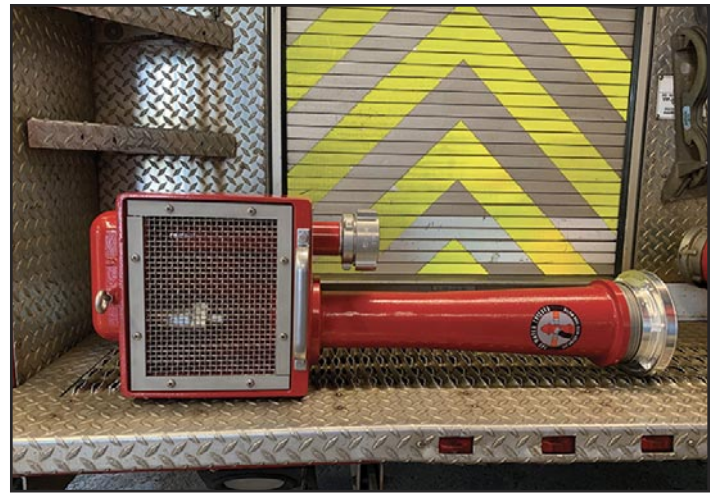
4 The TurboDraft Fire Eductor is equipped with a 2½-inch inlet that supplies the nozzle located within the basket strainer housing. This nozzle is pointed toward the volute, where a 5-inch return hose is connected that supplies the pumper with water.
