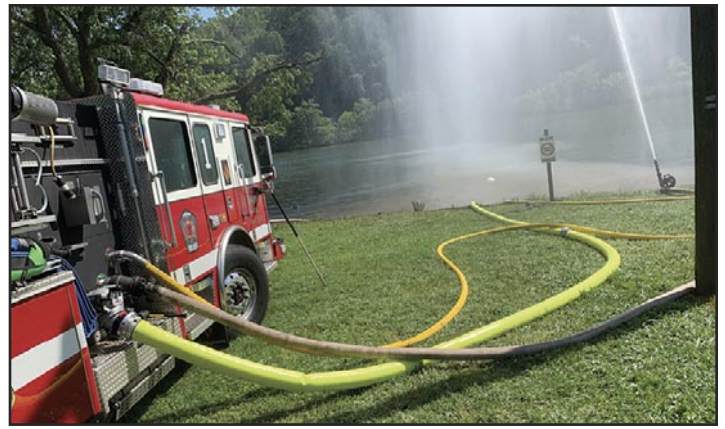
8 Once the discharge feeding the TurboDraft is opened, the operator will almost immediately notice water returning toward the pumper through the 5-inch supply line.
