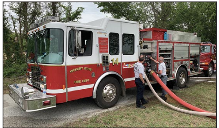
9 The operator must be mindful to maintain at least 200 psi on the discharge gauge supplying the device.
