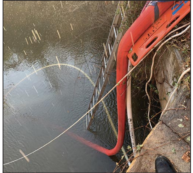
12 Kinks absolutely kill the return flow rate provided by the TurboDraft. In this photo, a backboard is used to remove the kink originally formed by the supply hose being laid over the corner of a bridge.
