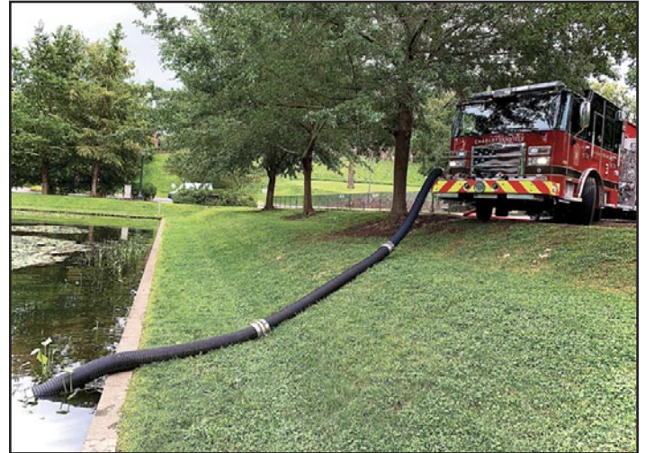
2 One option for reaching distant water sources is to perform “the long reach” using multiple sections of hard suction hose.
