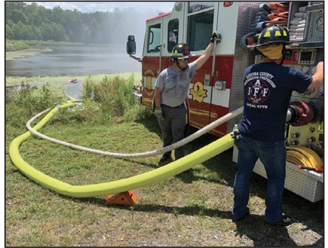
11 The minimum size return line that should be used during conventional TurboDraft operations is 5-inch hose.
