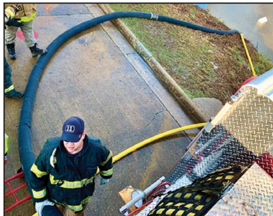
2 By switching out the 50-foot 5-inch return line with 50 feet of 6-inch soft sleeve, the flow rate from this single TurboDraft increased from 700 gpm to 950 gpm.
