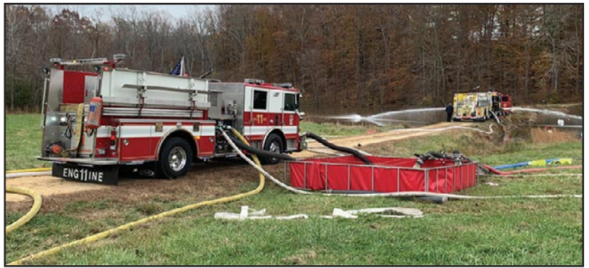
12 Using this advanced TurboDraft tactic allowed a third arriving fill site pumper to access the water source and increase the fill capability of the fill site without cramping the narrow levy that the other two pumpers were operating on. This configuration allowed the three pumpers to work in conjunction to support a 3,000-gpm fill site.
