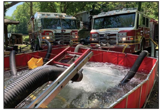
7 The engine on the right is supplying two TurboDrafts that are filling a dump tank that is 150 feet from the water source and 25 feet above the source. The engine on the left is drafting from this dump tank and flowing 1,000 gpm without outpacing the supply from the TurboDrafts. The engine on the right is able to maintain the flow to both TurboDrafts and keeps the tank full because it too is drafting from the dump tank to maintain the process.
