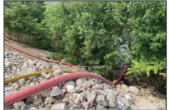
5 A tandem TurboDraft operation being employed to increase the operational flow capabilities over challenging terrain with significant distance and lift.
