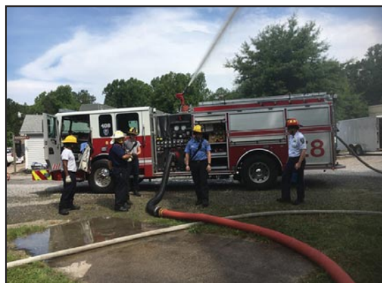
4 Hard sleeve being used by a Hanover County (VA) Fire Department engine to prevent a kink from forming at the intake from the weight of the supply line.
