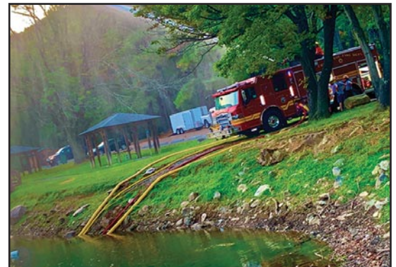
6 By employing a tandem TurboDraft operation, the flow capability of this pumper was increased to 1,000 gpm.
