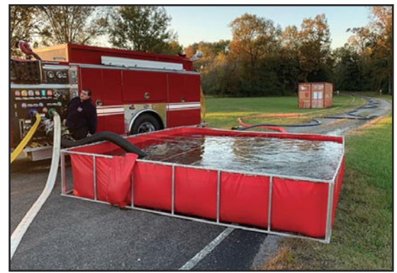
9 This engine is supplying a TurboDraft located in a creek 350 feet away and using the water from the device to fill a dump tank. The engine is then able to draft out of the tank and fill tankers at a rate of 1,000 gpm while also supplying the TurboDraft.
