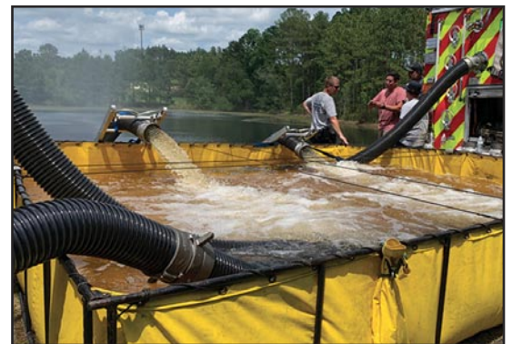
8 Tucking the hard sleeve from the TurboDraft return line between the last two rungs of a ground ladder allows the hard sleeve to act as a spout that directs water right into the tank.
