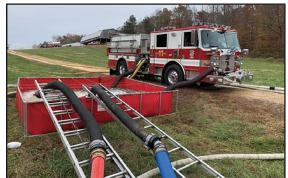
10 La Plata (MD) Fire Department Engine 11 supplies two TurboDrafts that are filling a dump tank from which the engine is drafting. By using two TurboDrafts to fill this tank, Engine 11 was able to fill tankers at 1,000 gpm without the risk of draining the dump tank.
