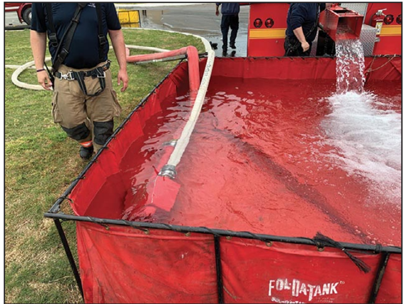
13 Flipping the TurboDraft upside down is an option for “clean bottom” shallow water sources and dump tank operations.
