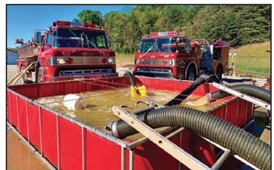
11 When resources allow, it is advantageous to use two pumpers for this TurboDraft tactic; one pumper will draft out of the tank and supply the TurboDrafts to ensure the tank remains full while the other drafts and supplies water where is needed.
