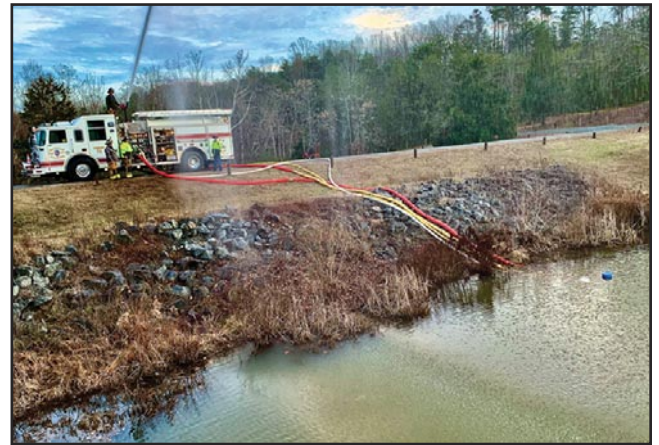
1 Employing a tandem TurboDraft operation allowed this Scottsville (VA) Fire Department engine to flow 1,000 gpm from a source 75 feet away. (Photos by author.)
