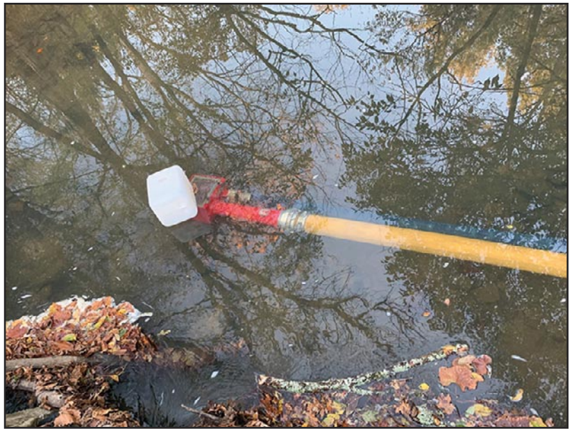
15 For shallow sources with silty bottoms, place the TurboDraft right side up with the return line run into a dump tank. The supply engine can then draft out of the tank.
