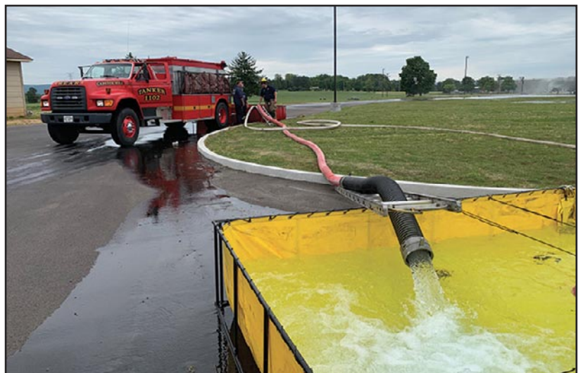
14 The TurboDraft in the far tank allows water to be easily transferred to the primary dump tank over a distance.
