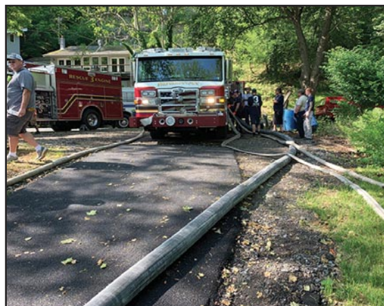
3 Fifty feet of 6-inch hose is being used by this Shepherdstown (WV) Fire Department engine to finish the layout from the TurboDraft that already has 100 feet of 5-inch attached.
