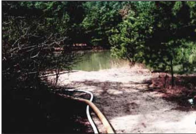
Due to soft sand and trees the engine was not able to be positioned to allow for drafting at this location. With the Turbodraft we were able to access the water source from approximately 100 ft away and fill tankers at a rate of 600 gpm.
