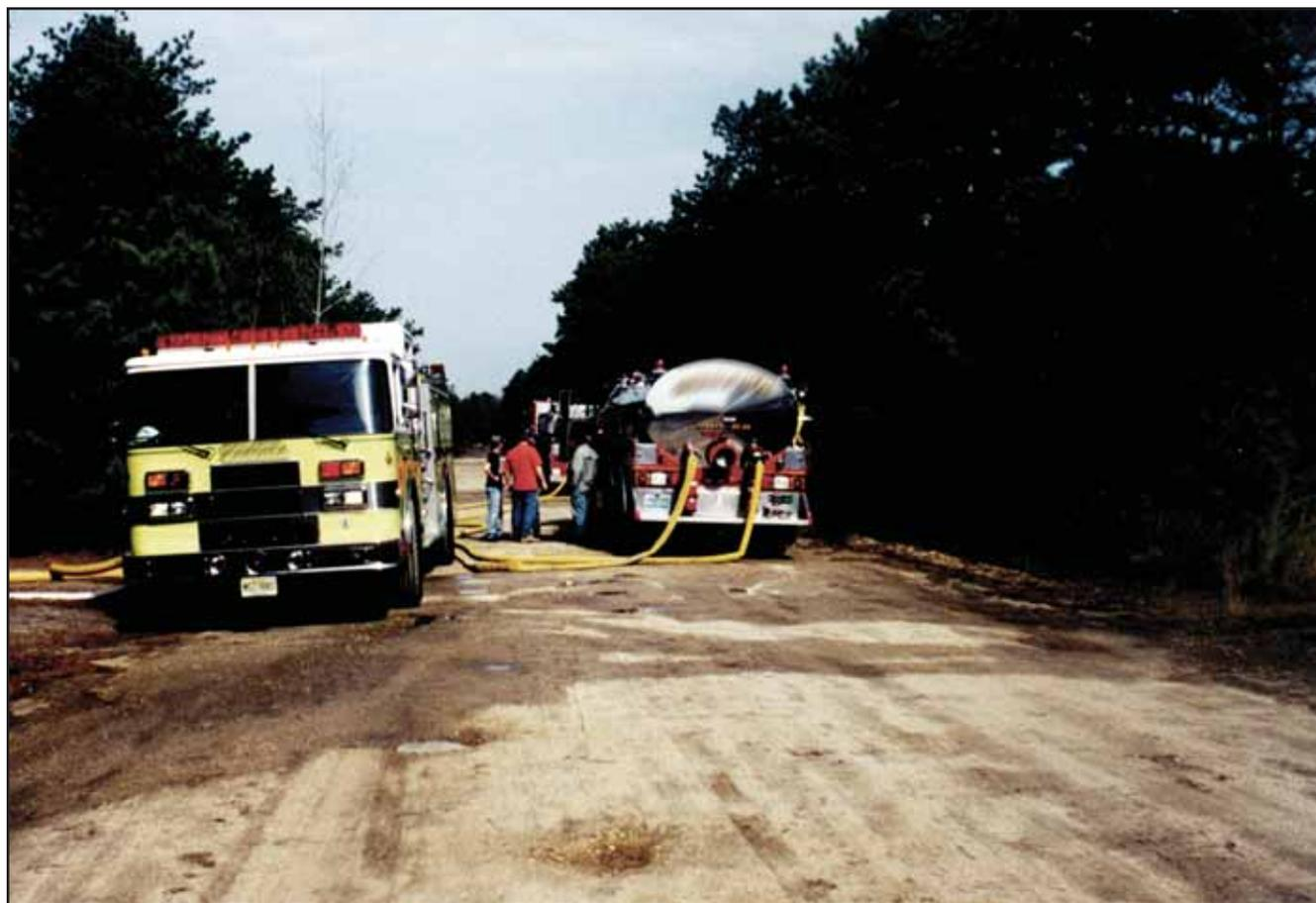
Tanker shuttle drill using TurboDraft at a fill site that was not accessible for typical drafting techniques.
