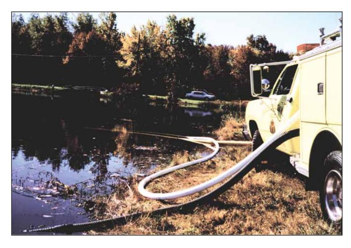
Drafting with a 300 gpm brush truck and supplying the Turbodraft with 200 gpm at 150 psig. This turned the brush truck into a water supply unit by sending the full 870 gpm of water out to the engine which is able to stay on the road.
