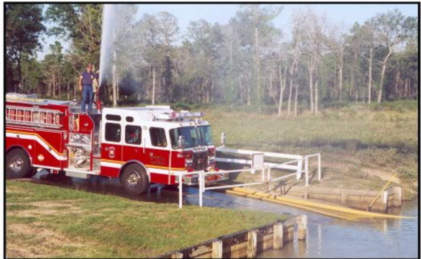
This 50-foot preconnected TurboDraft allows for drafting water 50 feet from the vehicle with a lift to 48 feet in less than two minutes with one firefighter.
