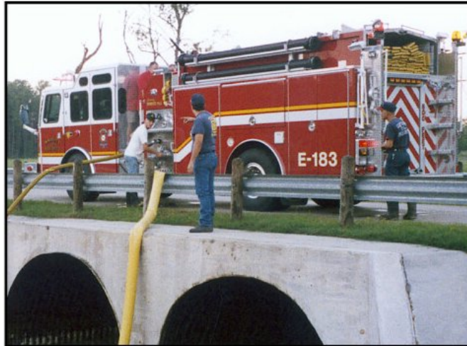
Excessively high lifts and long stretches that rule out drafting do not rule out the use of a TurboDraft
