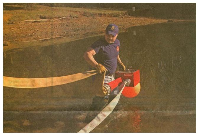
Henry Lovett of the Turbo Draft Co. gives a demonstration to volunteer firefighters at Rockwood Beach. The device can turn a body of water into a source for firefighters where hydrants may be limited or nonexistent.
