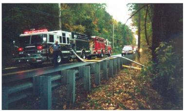
**Figure 10.** Due to a limited tanker shuttle area, firefighters dropped a TurboDraft into the Delaware Canal. The pumper in the foreground operated the TurboDraft and supplied the pumper in the background with water for foam standby lines.
