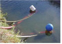
Figure 17. Here are two TurboDrafts equipped with floats to hold them off the bottom of the stream.
