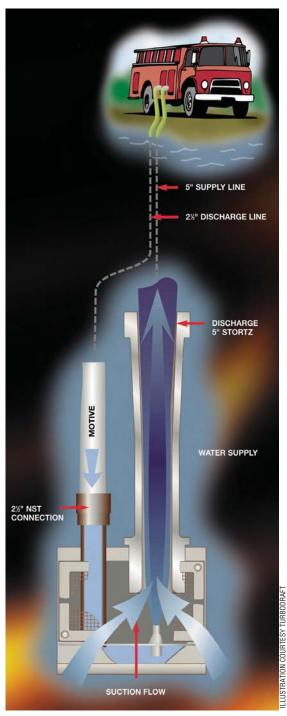
**Figure 2.** The design of the TurboDraft creates a venturi where the water from the 2½" line exits the nozzle and enters venturi tube. The venturi creates negative suction that draws additional water in through the strainer for discharge into the 5" line.
