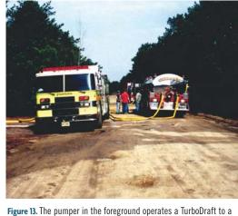
**Figure 13.** The pumper in the foreground operates a TurboDraft to a water source 100 feet to the left of the pumper, and it uses the excess water to fill tankers at a water shuttle fill site.
