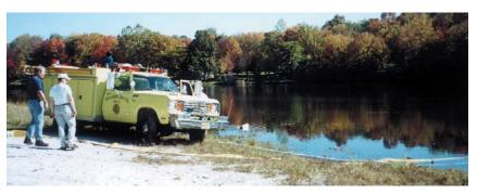
Figure 11. In this case, a mini pumper with a 300-gpm at 150-psi fire pump drafts from a water source to supply the TurboDraft. But instead of the 5" discharge line feeding the mini, the 5" line supplied a pumper on the main road.
