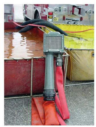
Figure 1. Here is the standard TurboDraft with 2½" and 5" hoselines connected. The 2½" or "motive" line supplies the water to operate the TurboDraft. The 5" line serves as the supply line from the TurboDraft to the pumper or other device. Depending on conditions explained in this article, a 200-gpm flow through the 2½" line can cause the TurboDraft to pick up an additional 800 gpm and deliver it through the 5" hose to a pumper or other device.
