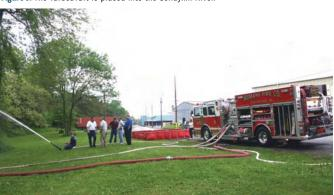
Figure 6. The Humane Fire Company's pumper supplies the TurboDraft through a  $2\frac{1}{2}$ " line, which in turn supplies the pumper with about 800 gpm through the 150-foot 5" line. The pumper then used the excess water to supply the portable monitor with more than 500 gpm.
