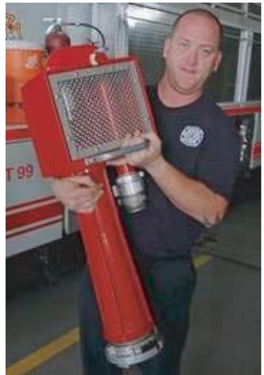
Malabar firefighter/paramedic Matt Clark holds the TurboDraft, which can pump water from rivers, lakes and ponds at a high rate.
