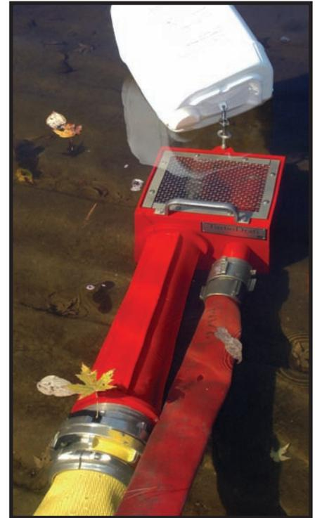
A TurboDraft is ready to be charged at a boat ramp on the Connecticut River. The attached pail provides buoyancy. Tank water from the apparatus is sent through the 2½-inch hose at about 180 psi to create suction in the 5-inch return line, providing a useable flow of up to 670 gpm.
