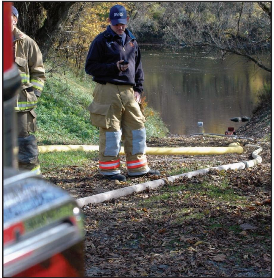
A lift of about 20 feet through 150 feet of hose was no challenge for the TurboDraft, which produced about 300 gpm of useable flow in this evolution.
