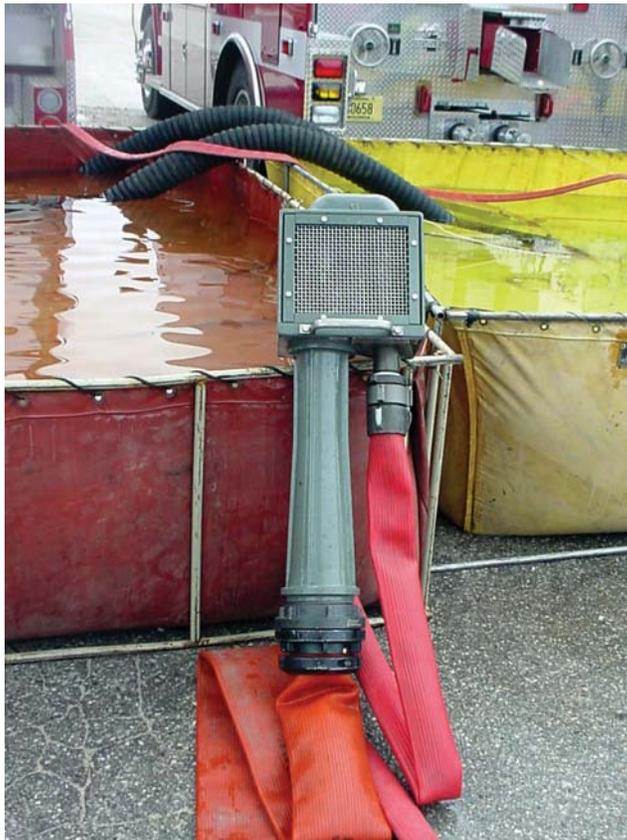
**Figure 1.** Here is the standard TurboDraft with 2½" and 5" hoselines connected. The 2½" or "motive" line supplies the water to operate the TurboDraft. The 5" line serves as the supply line from the TurboDraft to the pumper or other device. Depending on conditions explained in this article, a 200-gpm flow through the 2½" line can cause the TurboDraft to pick up an additional 800 gpm and deliver it through the 5" hose to a pumper or other device.
