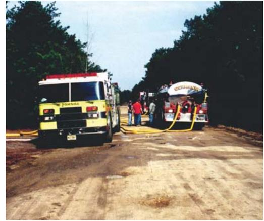
Figure 13. The pumper in the foreground operates a TurboDraft to a water source 100 feet to the left of the pumper, and it uses the excess water to fill tankers at a water shuttle fill site.
