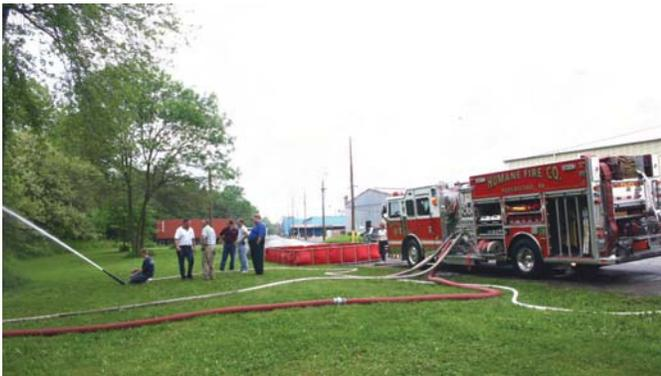
**Figure 6.** The Humane Fire Company's pumper supplies the TurboDraft through a 2½" line, which in turn supplies the pumper with about 800 gpm through the 150-foot 5" line. The pumper then used the excess water to supply the portable monitor with more than 500 gpm.
