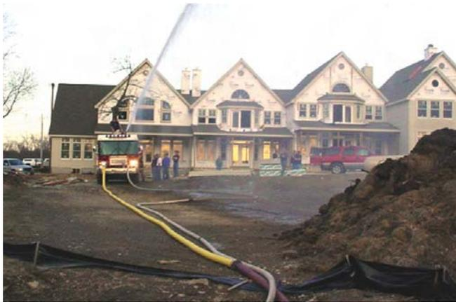
Figures 14 and 15 above: Here, the Fenton Township Fire Department operates a TurboDraft. The water source is a lake on which numerous condos have been built. The blue float holds the TurboDraft off the bottom, but about two feet below the surface of the water. Figure 14 shows the pumper, which has set up the TurboDraft and is preparing to discharge through its deck gun. Figure 15 shows the TurboDraft supplying the pumper with more than 500 gpm.
