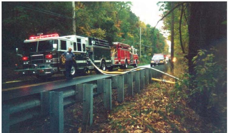
**Figure 10.** Due to a limited tanker shuttle area, firefighters dropped a TurboDraft into the Delaware Canal. The pumper in the foreground operated the TurboDraft and supplied the pumper in the background with water for foam standby lines.
