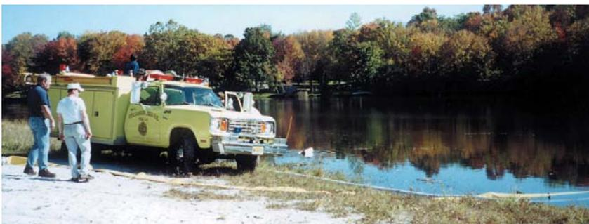
**Figure 11.** In this case, a mini pumper with a 300-gpm at 150-psi fire pump drafts from a water source to supply the TurboDraft. But instead of the 5" discharge line feeding the mini, the 5" line supplied a pumper on the main road.
