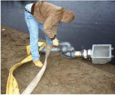
**Figure 3 above:** The original version of the TurboDraft was a modified marine eductor that Schutte and Koerting have manufactured for the Navy for shipboard firefighting for years. This test was conducted in Glastonbury, Conn.
