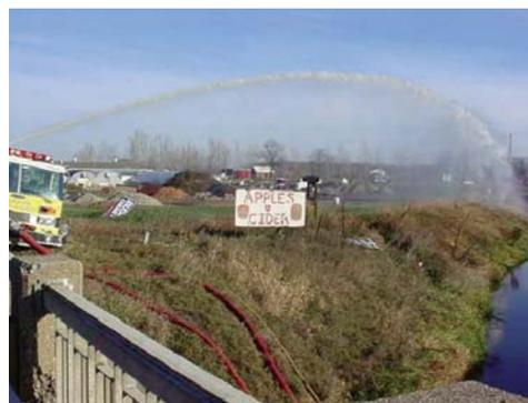
Figure 16. This department is using a single engine to supply two TurboDrafts (into a stream), which are supplying the pumper with a net flow of 932 gpm.
